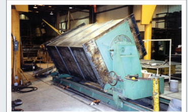
Jig welded for precise alignment
