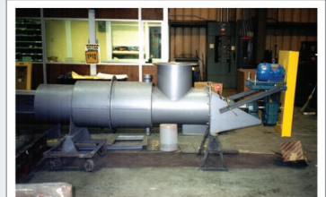
Water Cooled Injection Screw Conveyor
