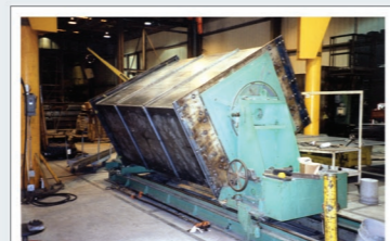
Jig welded for precise alignment
