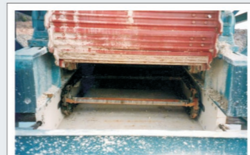
Clean-up Drag Conveyor
