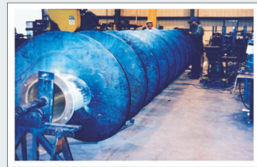
Large Diameter, Single Screw
